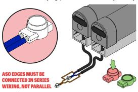
**8.** When joining cables between safety edges or junction boxes, use weather proof connectors such as gel crimps or properly soldered and heatshrinked connectors rated at IP 65 or above **!WARNING!** Failure to join cables properly will invalidate any warranty of the safety edge.
