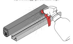
**4.** Use soapy water spray solution to coat the rubber foot and the alu carrier before attempting to install.
