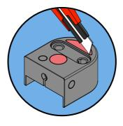
...remove both '**D' & 'O'** shaped drainage caps...
