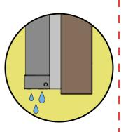
On vertical installations remove the drainage caps from the bottom end cap.
