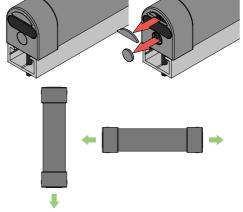
7. Finally ensure that water drains from the end caps have been removed as illustrated (for vertical installations remove only the lower water drain (for horizontal installations remove water drains from both ends of the safety edge) !WARNING! failure to remove water drains from the safety edge will invalidate any warranty.
