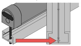
3. Drill additional 8mm hole in the desired location to draw any cables through the alu carrier and frame of gate/door.
