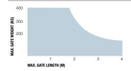
The shape, the height of the gate and the weather conditions can considerably reduce the values shown in the graph to the side.
