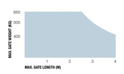
The shape, the height of the gate and the weather conditions can considerably reduce the values shown in the graph to the side. Use in windy areas 230 Vac models.
